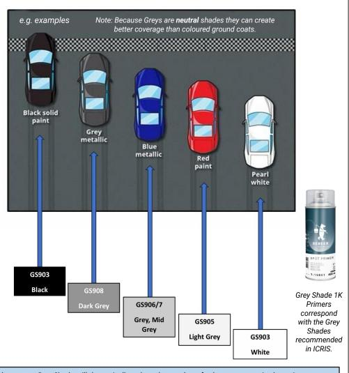
Using the correct Grey Shade will dramatically reduce the number of colour coats required to gain coverage over repairs. This can reduce paintshop costings in both time and product.
